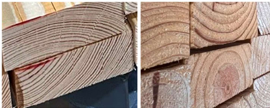
Figure 1: Comparison of growth rings in Missouri grown natural forest shortleaf pine lumber vs. plantation grown shortleaf pine lumber.
